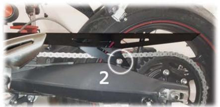
UNINSTALL THE ORIGINAL CHAIN COVER AND REAR FENDER REMOVING THE FIXING SCREWS ON THE REAR FORK (SEE THE PICTURE).
