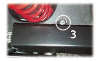
REMOVE THE REAR FENDER AND UNSCREW THE FIXING POINT OF CHAIN COVER (3).
