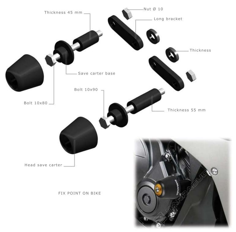
BEFORE BEGINNING THE ASSEMBLING PROCEDURE, LOCATE THE MOUNTING POINTS ON THE BIKE, USE THE SHIMS AND BOLTS AS DESCRIBED IN IMAGE IN ORDER TO GET THE RIGHT PROJECTION OF THE BUFFER FROM THE BIKE.
