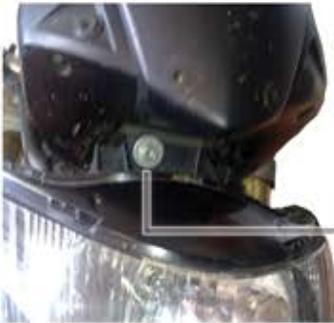
REMOVE THE CENTRAL FIXING SCREW OF HEADLIGHT AND LOOSEN THE TWO SCREWS ON THE SIDES
