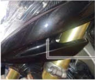
REMOVE THE HEADLIGHT-COVER UNLOCKING THE TWO SCREWS ON THE SIDE
