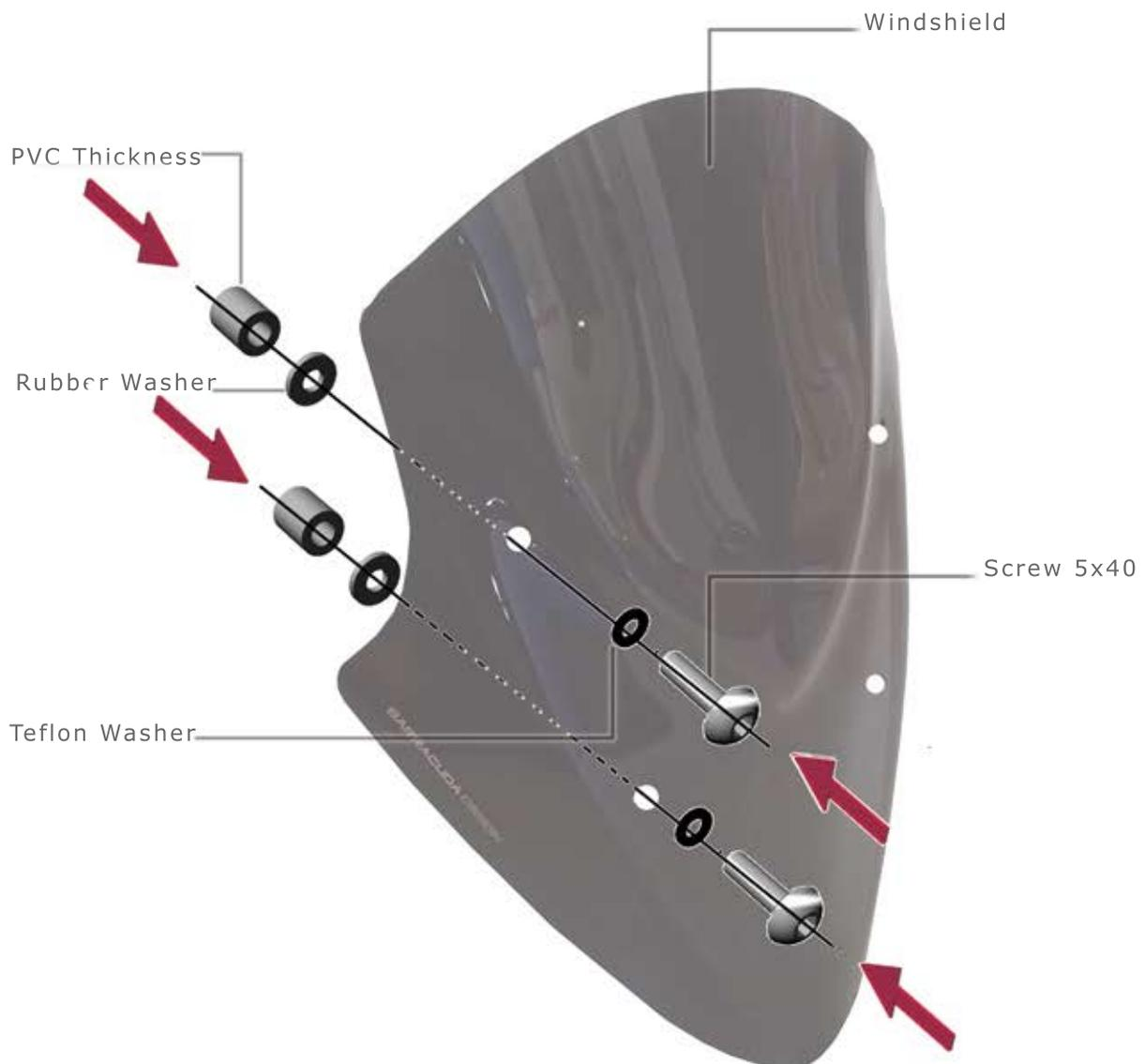
REMOVE THE 4 FIXING SCREWS OF THE ORIGINAL WINDSHIELD, MOUNT THE BARRACUDA WINDSHIELD/SCREEN WITH THE SPECIFIC THICKNESS LIKE DESCRIBED UP.
